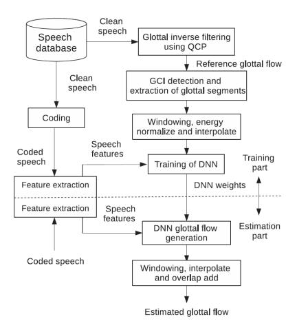
DNN-based estimation of the glottal flow from coded speech.
