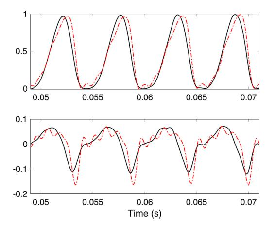
Examples of glottal area A (black curve) and glottal flow U (red curve) waveforms (upper panes) and their corresponding derivatives (lower panes) demonstrating skewness.
