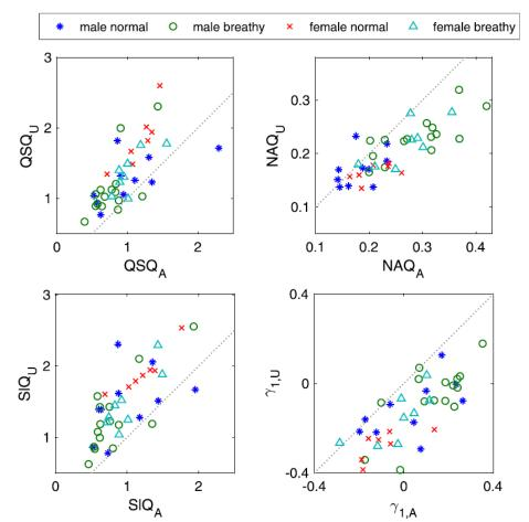
Values of four skewness parameters, extracted from both the glottal area (subscript A) and flow (subscript U) waveforms. Line y=x is shown for reference. Flow skewing manifests itself in dots that are located **above** the line in the parameters on left and **below** the line in the parameters on right.
