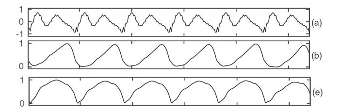
Distortion of the glottal flow when the input is coded telephone speech: (a) speech, (b) glottal flow estimated from clean high-quality speech, (c) glottal flow estimated from telephone speech.
