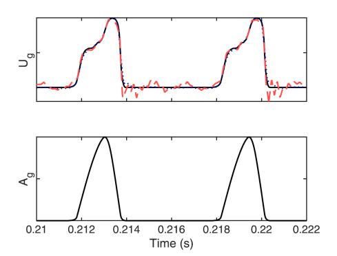
Top panel: Reference glottal flow (solid), as well the glottal flows estimated using two GIF methods (dashed, dotted). Bottom panel: Area of the glottal opening.
