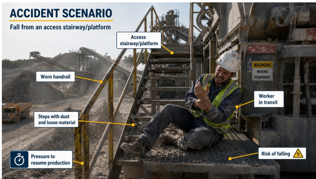
Figure 26. Scene of the accident on the stairway and access platform leading to the crushing area.
