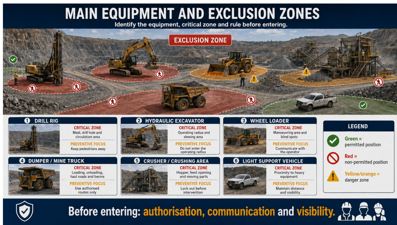
Figure 3.3 — Main equipment and exclusion zones
