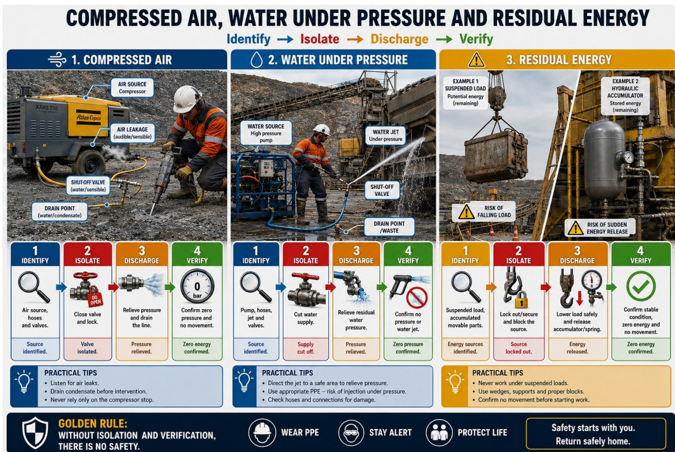
Figure 4.8 — Compressed air, pressurised water and residual energy
