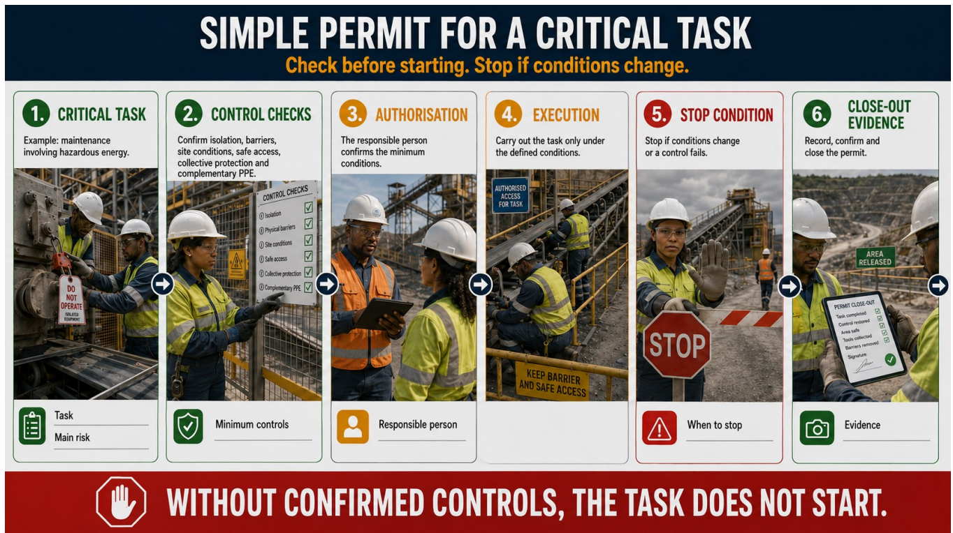
Figure 7.3 — Simplified permit-to-work for a critical task
