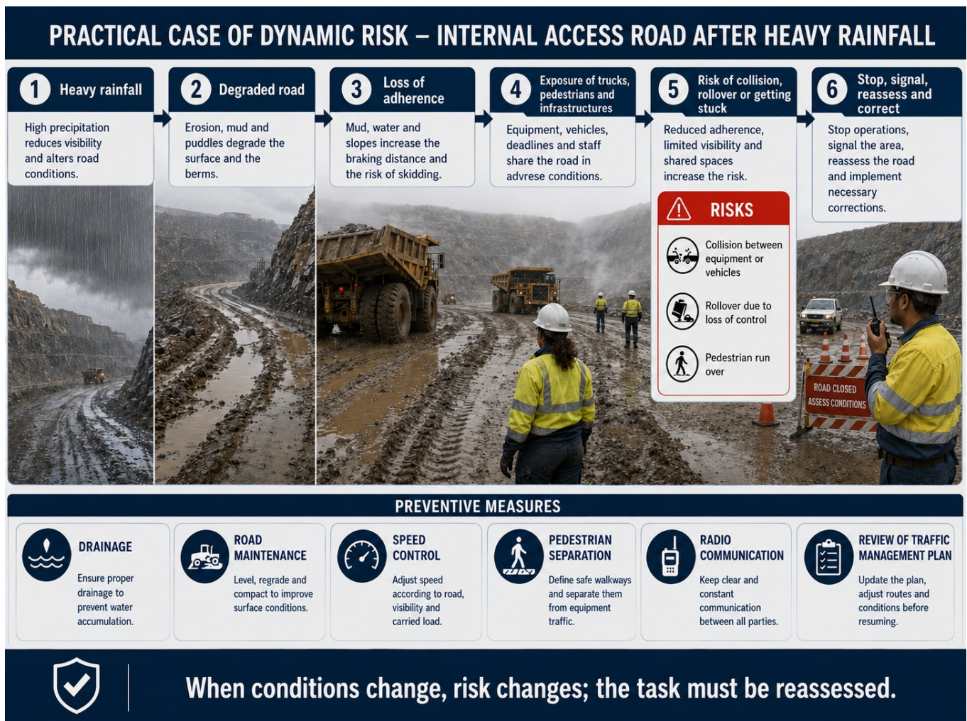
Figure 1.13 — Integrative case: dynamic risk on a deteriorated mine road after rain
