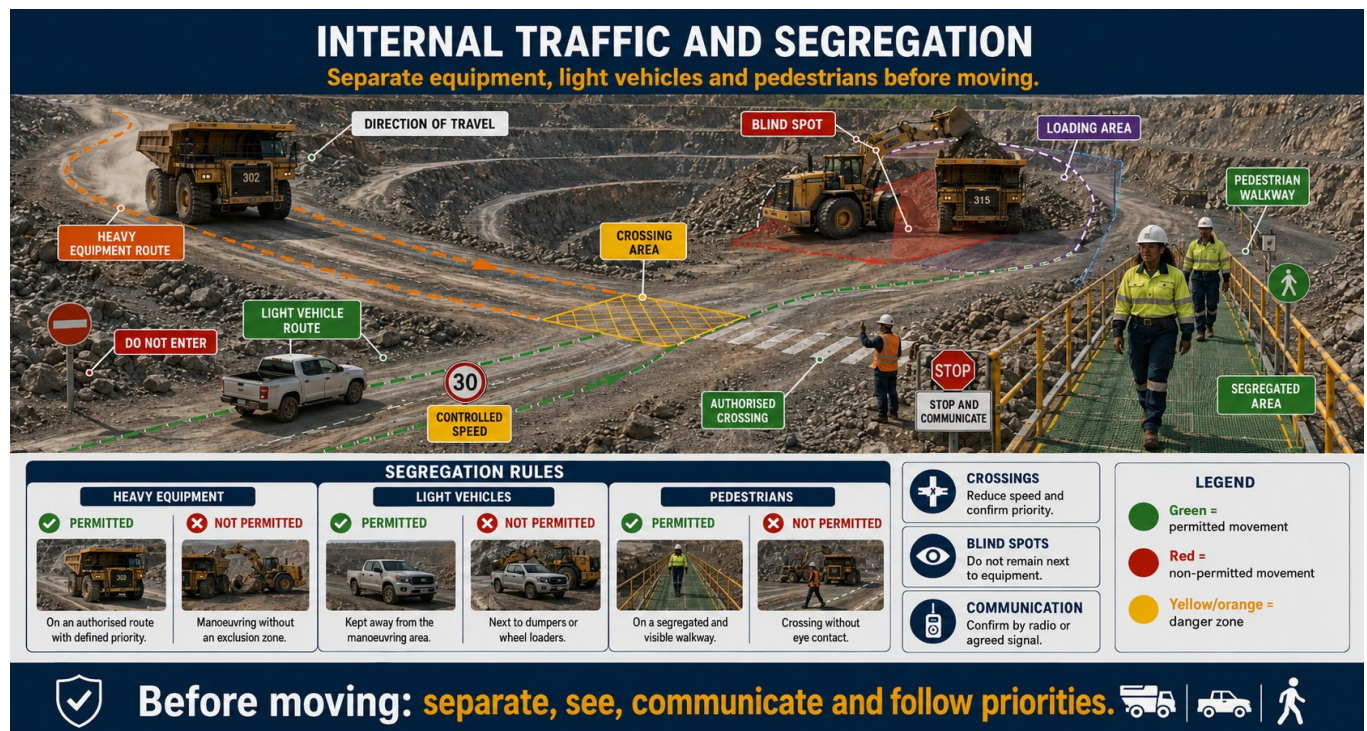
Figure 3.4 — Internal traffic and segregation between heavy equipment, light vehicles and pedestrians
