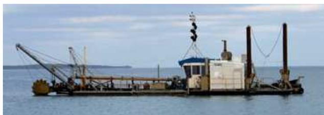
Figura 13. Bucket-wheel (<http://www.gendredge.com/nigeria/bucket.php>).
