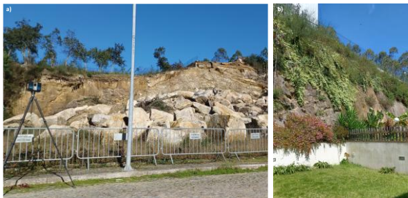
Fig. 4 a) Photo of the FARO Focus S350 Laser Scanner surveying the front of the slope; b) Position of some spherical targets.
