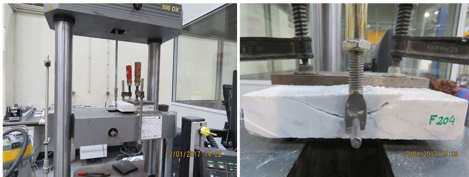
Fig. 7 - Examples of lab tests (breaking load at the dowel hole)
