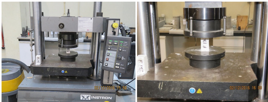
Fig. 6 - Examples of lab tests (compressive strength)
