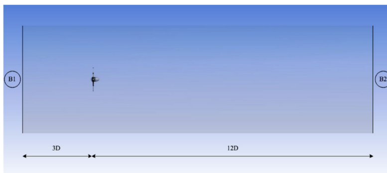
Fig. 4 - Computational domain specifications, WT distance relative to velocity-inlet (B1) and with pressure-outlet (B2)
