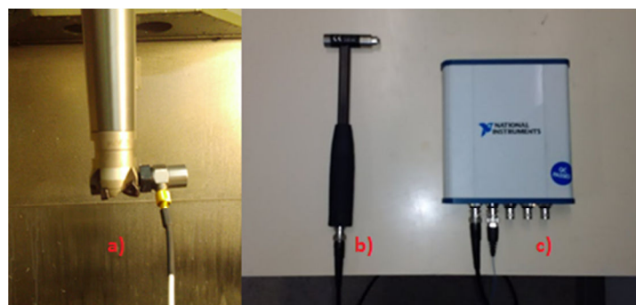
Fig. 1 - Instrumentation for measuring own frequencies (a) Accelerometer (b) PCB 86C03 and (c) NI 4431 USB.
