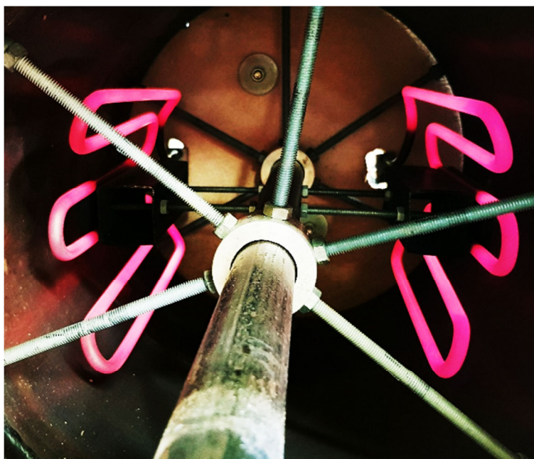
Fig. 1 - Interior of the pipe with electrical resistance heating.
