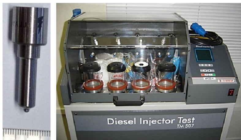
Fig. 1 - Test rig Diesel Injector Test TM 507 Common Rail
