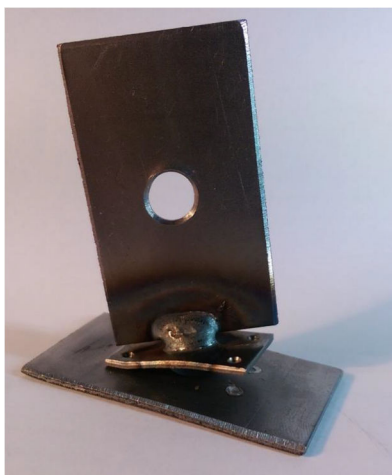
Fig. 1 - Specimen after tensile test
