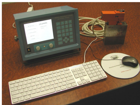
Fig. 1 - Ultrasonic Computerized Complex for residual and applied stress measurement UltraMARS-7
