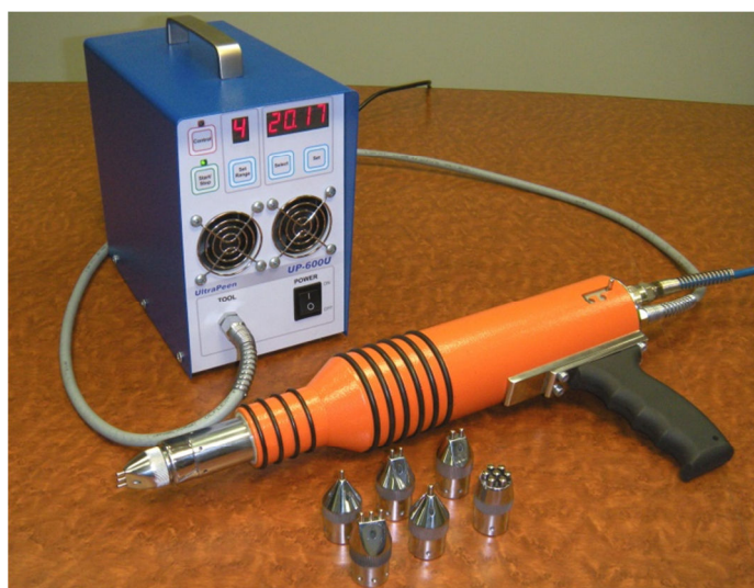
Fig. 1 - Ultrasonic impact treatment system for fatigue improvement of welded elements and structures
