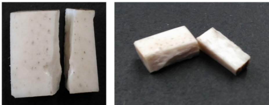
Fig. 11 - Cortical bone sample after brittle fracture
