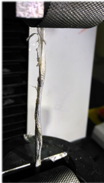
Fig. 4 - Tendon during tensile test
