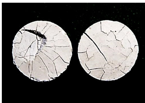
Fig. 1 - Degradation of ceramics based on zirconia in condition T=250^\circ\text{C} .
