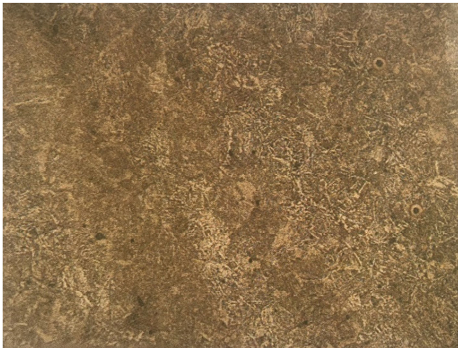
Fig. 1 - Microstructure of AISI4140 utilized to manufacture the crankshaft in this study (magnification 200X)
