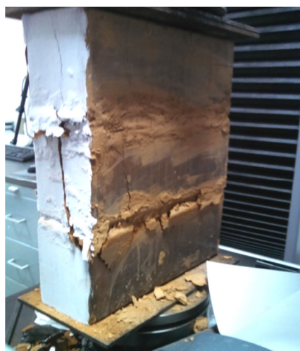
Fig. 5 - Typical failure mode of triplet compression test with CEB stabilized with 6 % cement.
