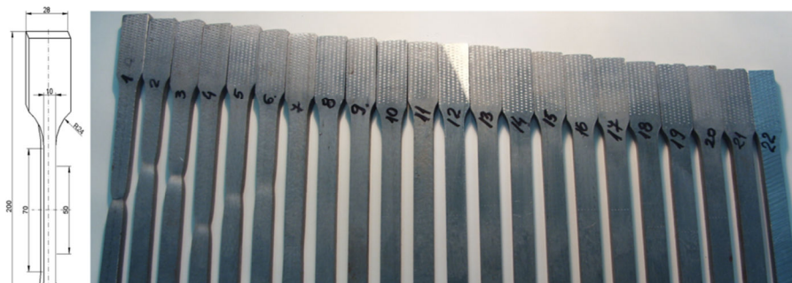
Fig. 3 - The 1C45 (1.053) steel specimens subjected to strain, in various stages of plastic strain
