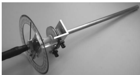
Fig. 12 Tracer gas injection device prototype.
