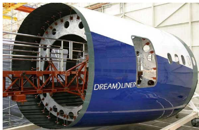
Figure.2. A Boeing 787 frame, tubular cylinder composite (Freissinet, 2011)
