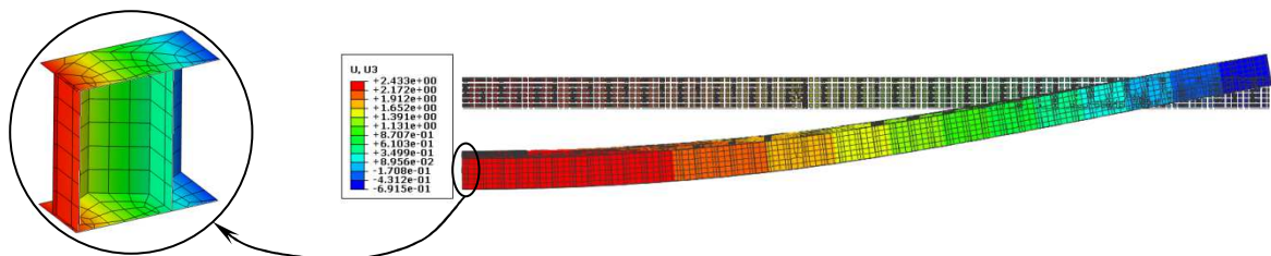
Fig.12 Deflection of beam under four-point bending load
