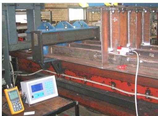
Fig. 1 - The process of residual stress measurement during fatigue testing of welded panel
