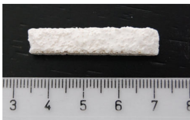
Fig. 7 Dimensional variation test specimen (5x40 mm, with thickness varying from 5 to 7 mm) cut from flexural strength samples
