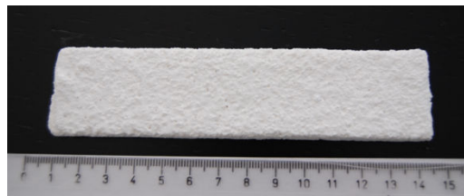
Fig. 5 Flexural test specimen (20x140 mm, with thickness varying from 5 to 7 mm) obtained in a wax mold
