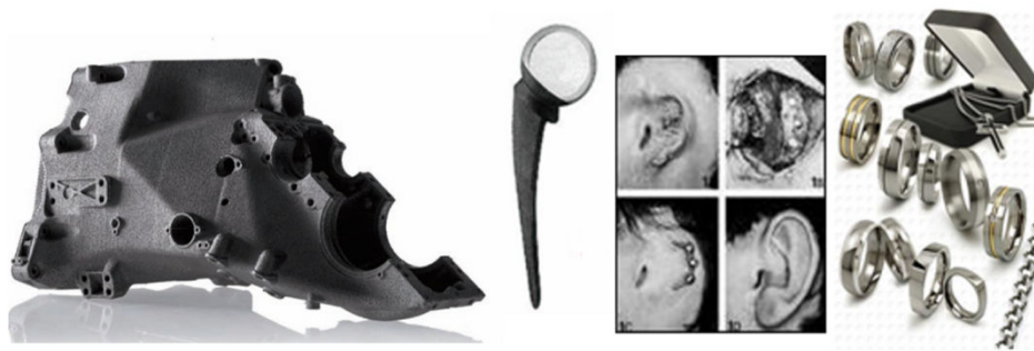
Fig. 1 Examples of applications of Ti and Ti alloys parts; from left to right: aeronautic component, medical implants, jewellery artefacts and accessories
