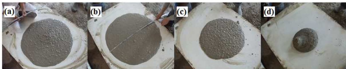
Fig 4: The influence of mixing time on slump flow.
