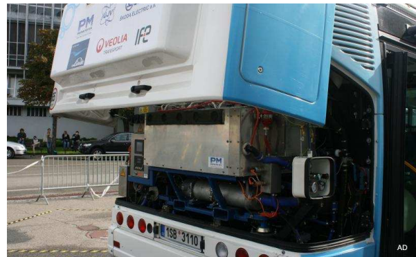
Fig. 2 PEM fuel cell in the back of the TriHyBus
