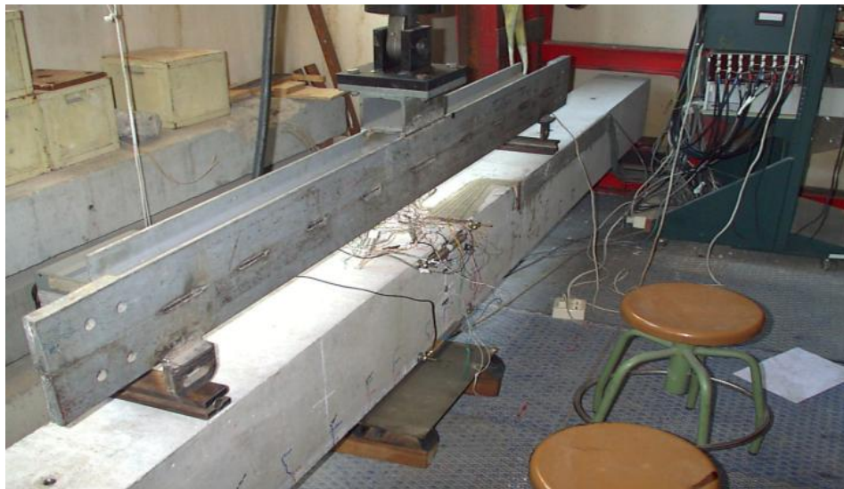
Fig.5 Tested concrete beam in structures laboratory of E.T.S. Ingenieros Industriales of Madrid
