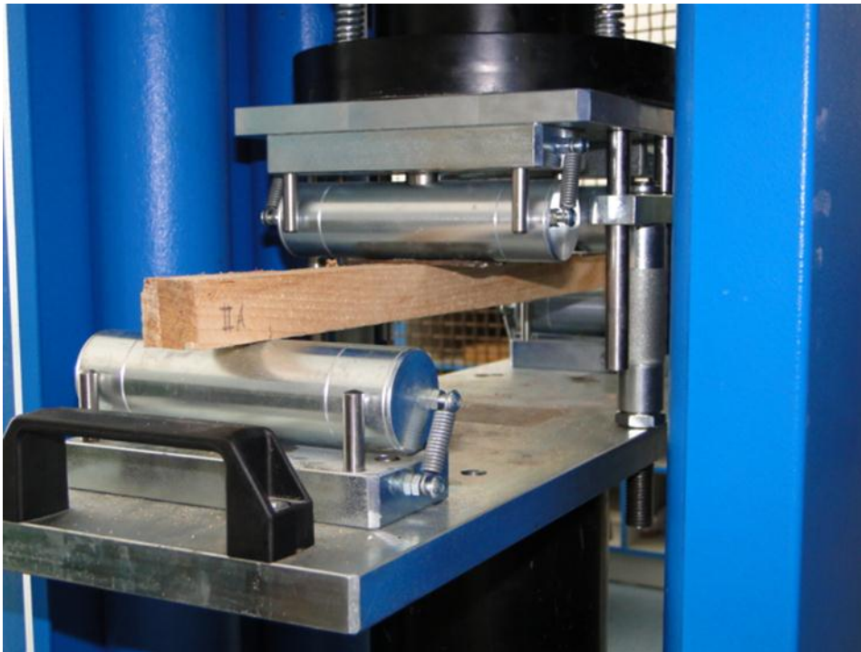
Figure 6 - Testing the bending strength
