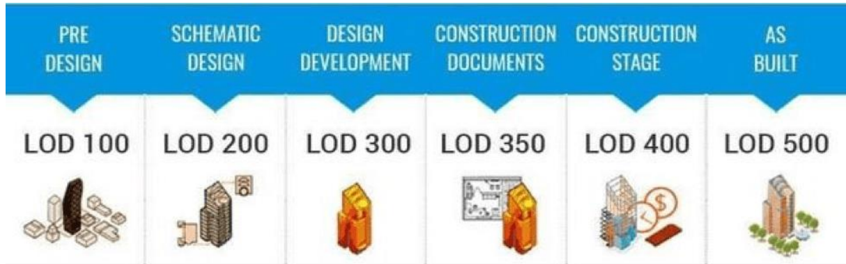
Figure 3.LOD levels and project stages. Source:[22]
