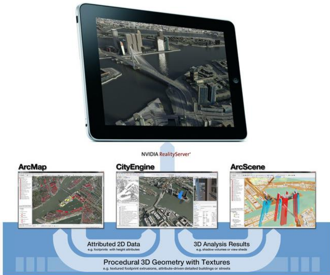
Figure 7. CityEngine Data Flow [37].
