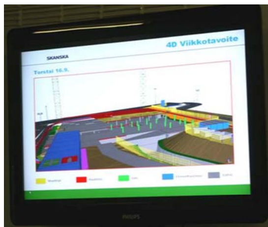
Figure 6. Example of slides in a presentation showing 4D-model views presenting the weekly plans.
