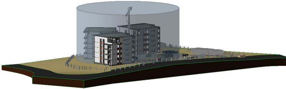
Figure 16. Visualization of crane reach (Sulankivi et al. 2009b).
