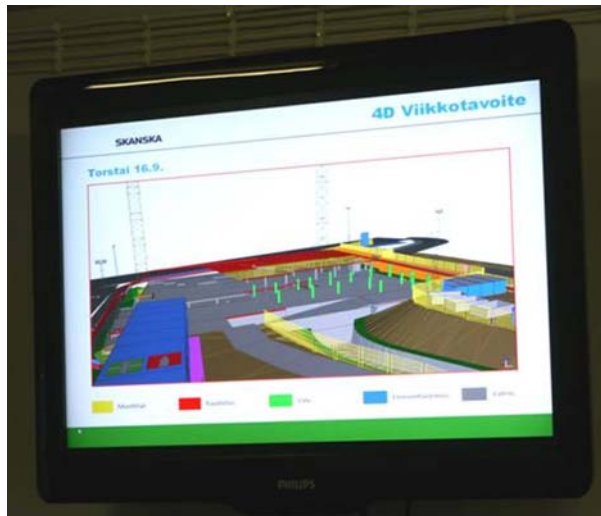
Figure 61. Example of slides in a presentation showing 4D-model views presenting the weekly plans.
