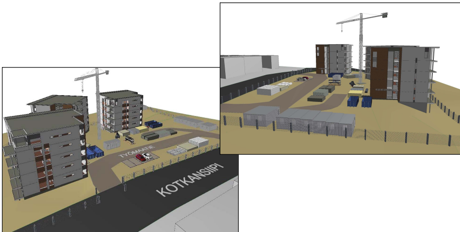
Figure 13. General views of the BIM-based site plan created using architectural modelling software ArchiCAD in the previous TurvaBIM research project.
