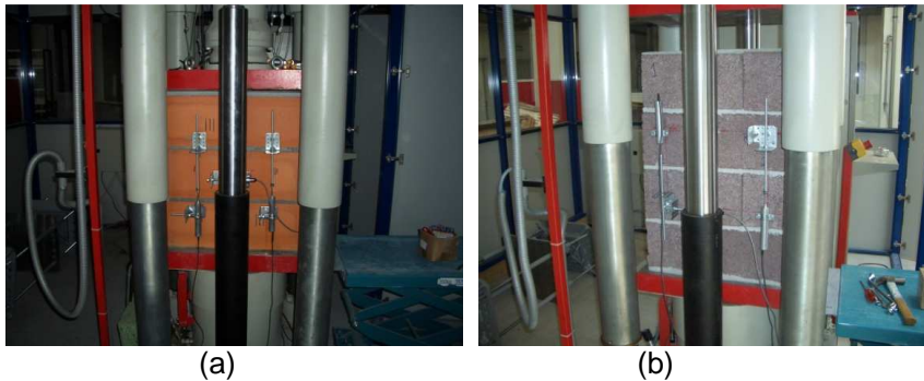
Figure 5. Example of compressive test set-up: (a) clay and (b) lightweight concrete masonry
