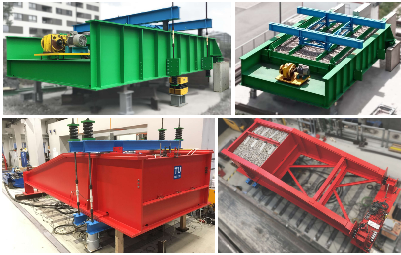
Fig. 7. Large-scale test facilities for isolated research of energy dissipation in the ballast superstructure: facility for investigation of longitudinal track-bridge interaction (top) and facility for investigation of vertical track-bridge interaction (bottom)
