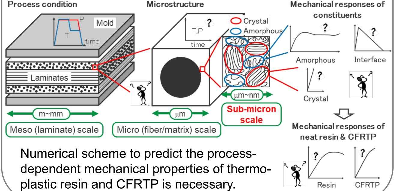
**Objective:** To establish a multi-scale & multi-physics simulation scheme bridging from process conditions, through crystal structure, up to mechanical properties of thermoplastic resin and its composites.
