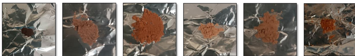
Figure 1. Different Zn-MIL53(Fe)-based MOFs, from left to right (ratio Fe:Zn): 2:3, 3:1, 1:3, 1:1, 1:2 and 2:1.
