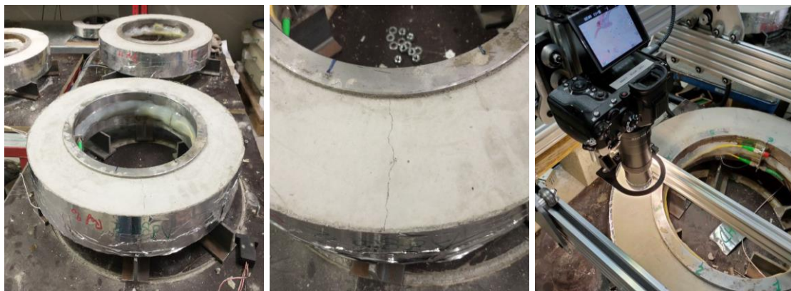
Figure 5. Restraint concrete shrinkage ring test setup.
