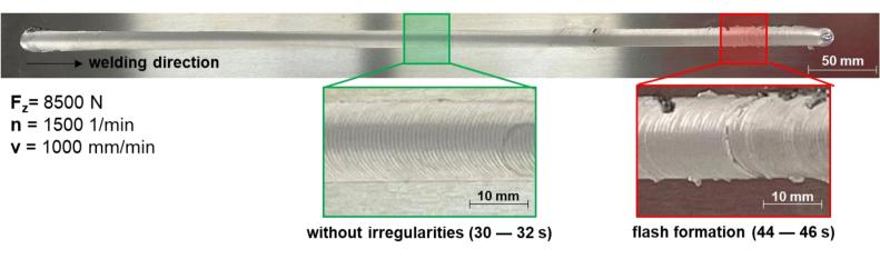
Figure 6: Varying surface quality at the center and end of the weld seam
